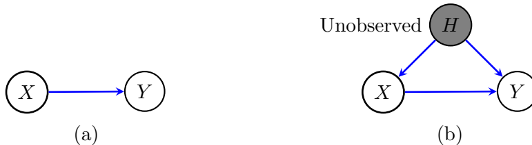
Figure 1: (a) A causal DAG representing two unconfounded variables; (b) A causal DAG representing the presence of confounding.
